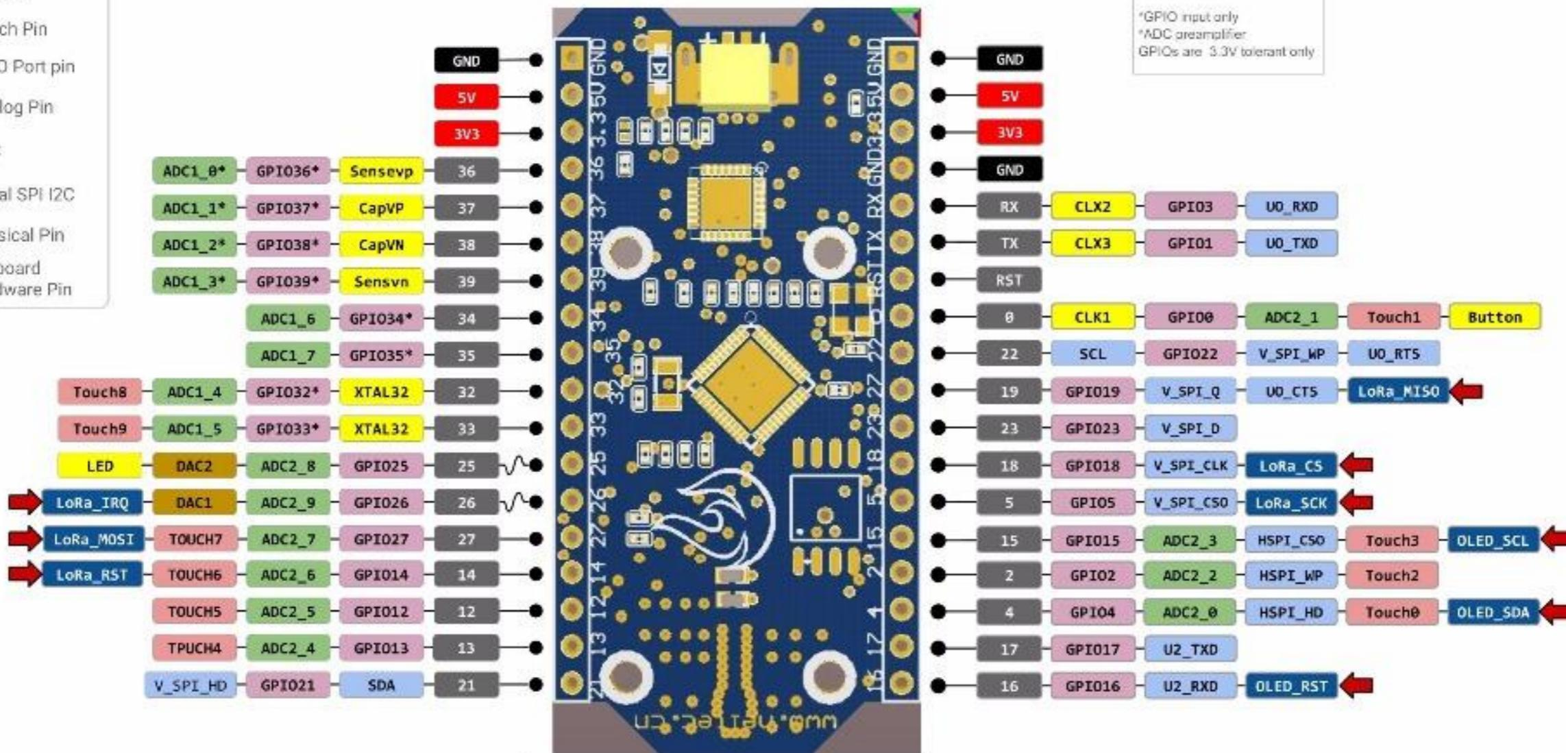
→ Pins with this arrow are used by on-board OLED or LoRa, they must not be used for other purpose unless you know what you are doing!
